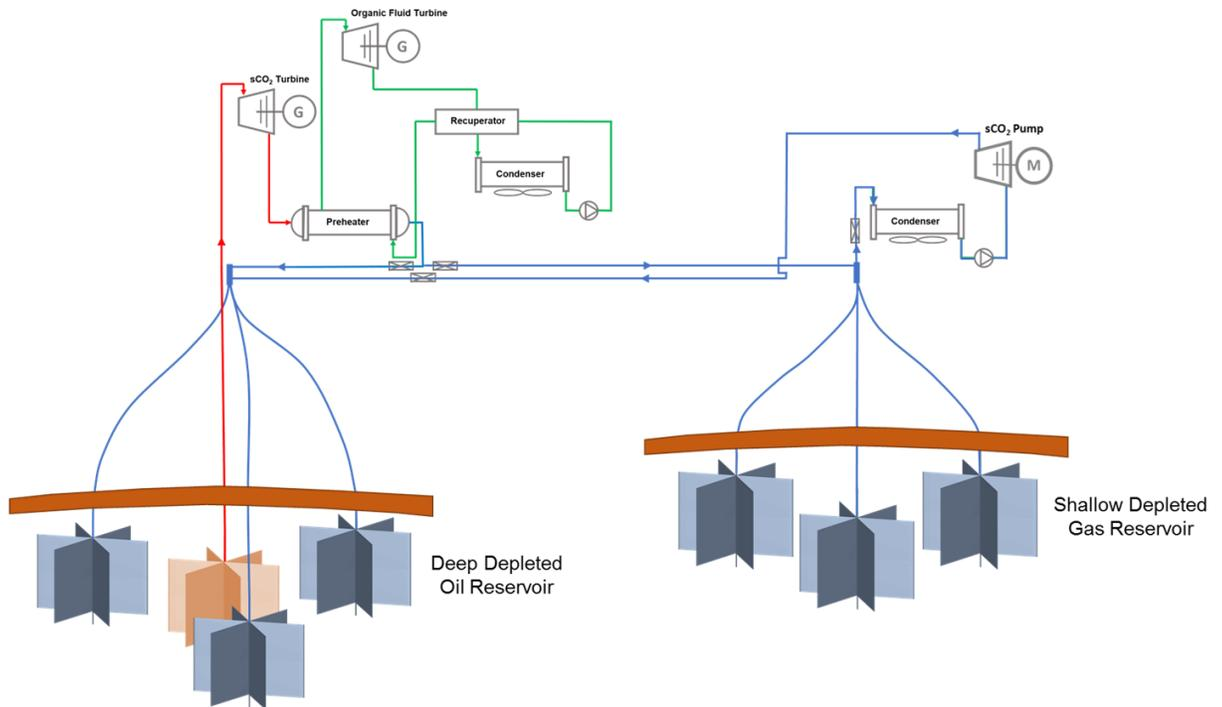
**Figure 2. Schematic of Subsurface Carbon Energy Storage Scheme, with the Dynamic Capability of Modifying the Storage/Generation Capacity.**
