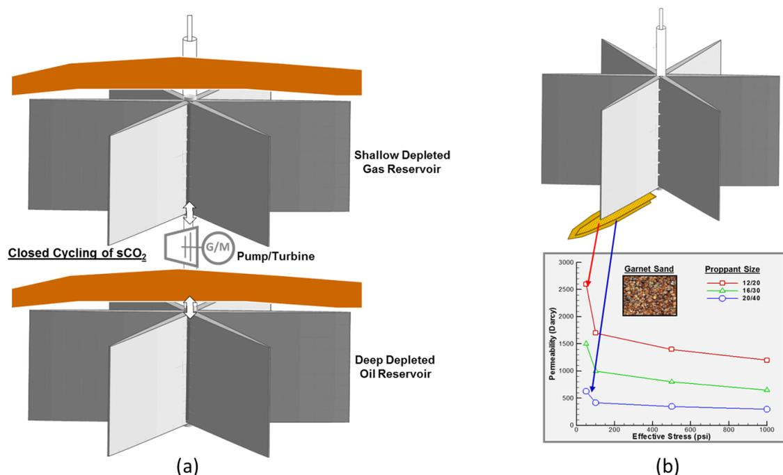
**Figure 1. Subsurface Carbon Energy Storage, a) Closed Cycling of Supercritical Carbon Dioxide between Shallow and Deep Reservoirs, and b) Multi-Azimuth Garnet Sand Propped Well.**
